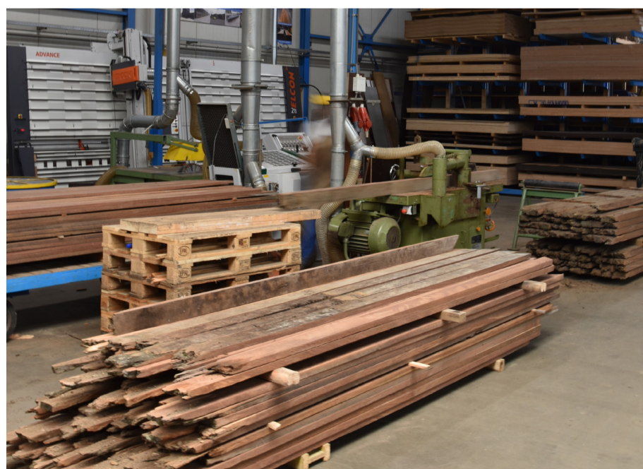
When the old Dutch quay walls are replaced for a new quay wall, the wall and its wood are taken apart and transported to be processed for a second life
